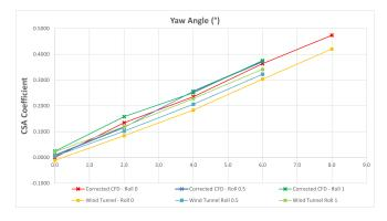
Figure 17: CSA against Yaw angle @ 16m/s air velocity and different roll angles
