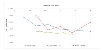
Figure 14: CDA against Air Velocity - Comparison between initial and corrected CFD models, and experimental data
