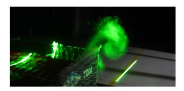
Figure 12: Smoke and laser visualization of the rear endplate vortex
