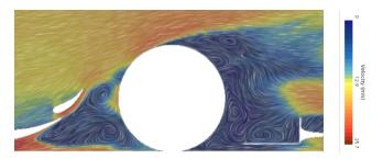
Figure 6: Wheel Wake around MANIC-24's wheel in track conditions
