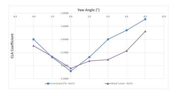
Figure 15: CLA against Yaw angle @ 16m/s air velocity and neutral roll
