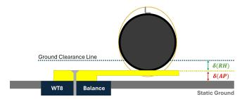
Figure 8: Schematic of the 2023 WT8 situation with increased ride heights
