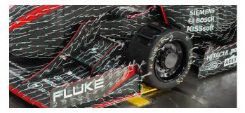
Figure 5: Wheel Wake Turbulators on DELTA-25's Front-Left wheel
