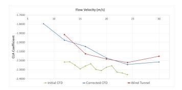
Figure 13: CLA against Air Velocity - Comparison between initial and corrected CFD models, and experimental data
