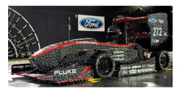
Figure 4: DELTA-25 with wheel wake replication devices and ground clearance adjusting wheels strapped to WT8 balances with FSAE adapters
