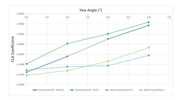
Figure 16: CLA against Yaw angle @ 16m/s air velocity
