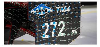
Figure 11: Tufts arranged to capture the boundary layer separation on the rear wing endplate of DELTA-25
